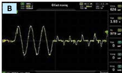
Graph B (at left) indicates startup of a typical RV air conditioner receiving power through a SoftStartUp module. The power spikes are quickly reduced to eliminate stalled A/C, RV power cutoff, premature A/C compressor failure, and other problems associated with A/C startup.
